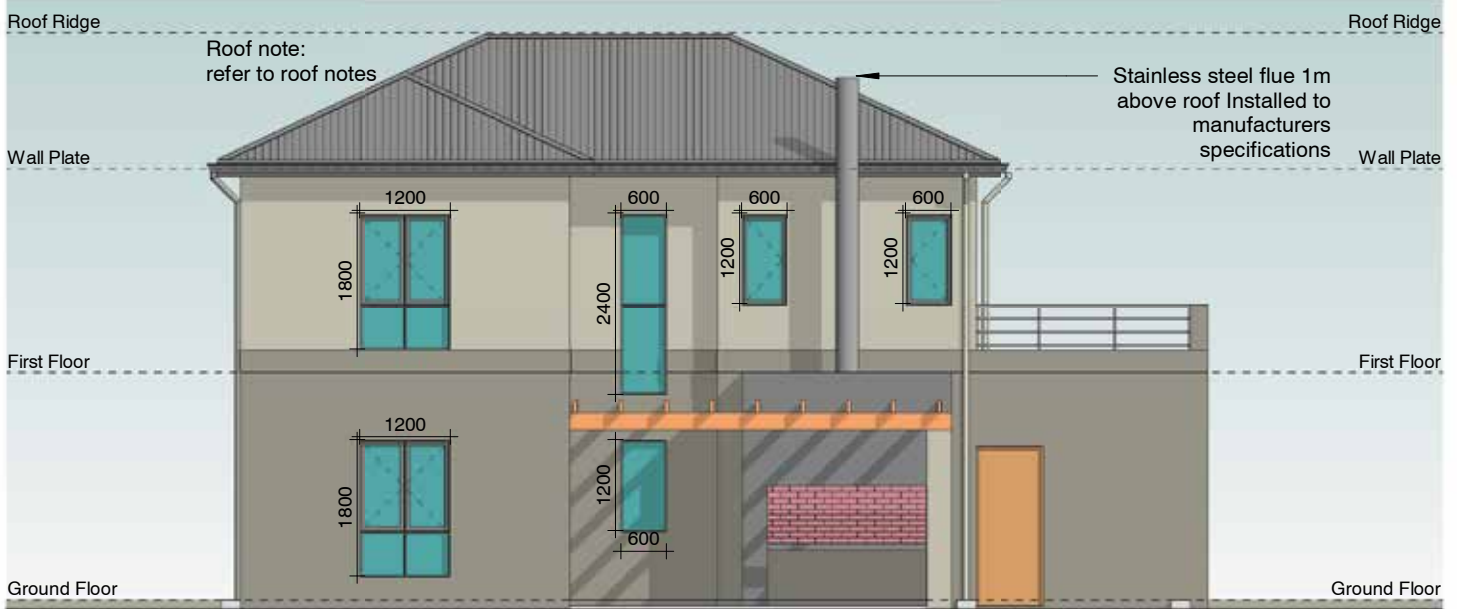
North Elevation (House 02) Scale 1:100
